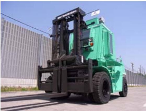
[Special heavy-duty forklift with radiation shielded cabin]
